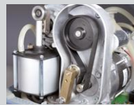
Flat belt drive of a suction pump
