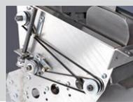
Drive unit of a friction feeder
