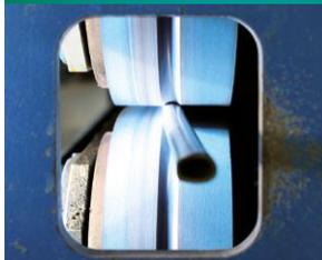
These endless haul-off belts are used in all kinds of machines, e.g. in caterpillar haul-offs for cables, wires, pipes, hoses, profiles, plastic foils, etc.
